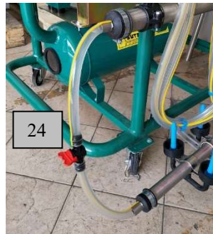
Wash line valve
